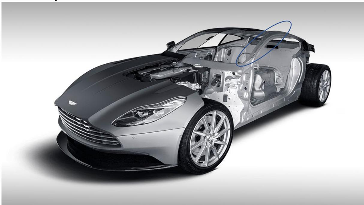
Aston Martin is one of the first OEMs to realise the benefits of designing parts using HFQ<sup>®</sup> Technology. The desire to reduce overall weight and part complexity, but enhance torsional rigidity and structural integrity, allowed designers and engineers to work with HFQ<sup>®</sup> Technology from the earliest phase to design, prototype and manufacture a new A-pillar pressing without compromise.
