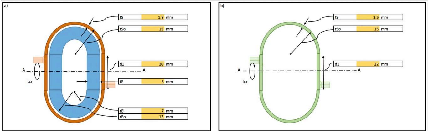
**Figure 2a (left) and 2b (right):** Simplified A-pillar cross-sections to identify relative performance of conventional vs HFQ<sup>®</sup> design solution. Flange details (shown as light horizontal extensions) were not considered in the calculations.
