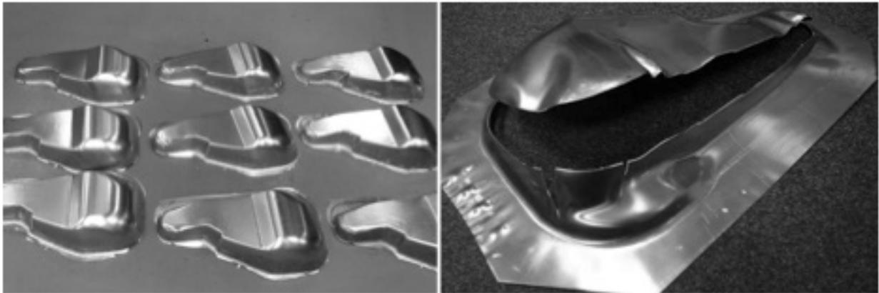
**Image 1:** (Left) Selection of successfully pressed deep-drawn rear bulkheads formed using AA6082 T6 aluminium with HFQ® Technology. (Right) Identical material and bulkhead part sheers when pressed at room temperature using conventional cold pressed methods.
