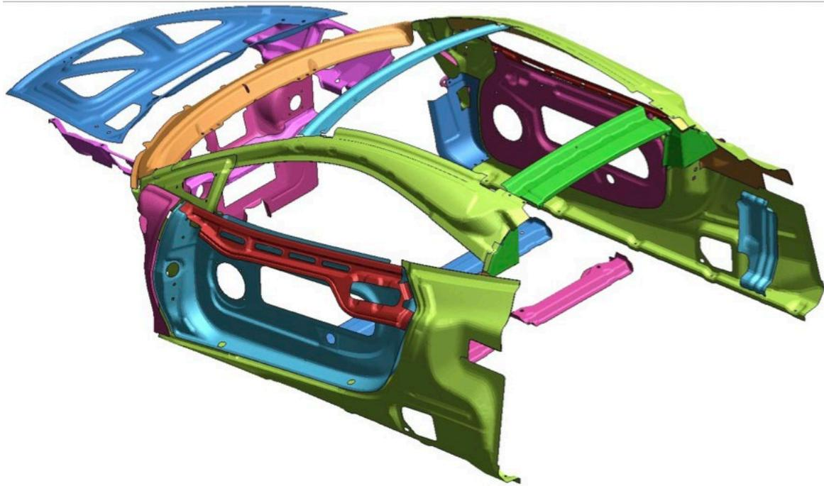
**Image 2:** Examples of components considered for HFQ<sup>®</sup> forming (reproduced from [3]). Colours used for clarity of individual parts.
