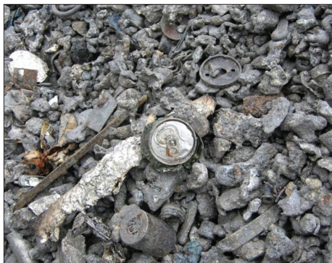
Figure 6. Bottom ash from domestic waste incineration contains the remnants of packaging and is often reprocessed for low-grade aluminum structures. HFQ tests on 6xxx sheet produced from near 100% bottom ash are an early demonstration of the potential to use this low carbon feedstock for structural aluminum applications in vehicles.
