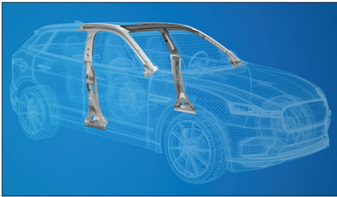
Figure 3. An HFQ safety cell representation based on the design used in the DBX. (Source: Impression Technologies.)
