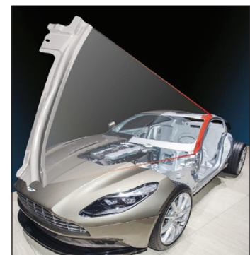
Figure 2. A narrow high strength A pillar formed by HFQ in 6082 alloy on the Aston Martin DB11.
