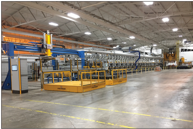
Figure 4. The hot forming line at Telos Global in Tennessee used for HFQ production trials in 7xxx series alloy.
